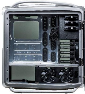
**Hybrid Metal Structure** – The case is made from a steel frame added with an aluminum motherboard tray and partition plate for a premium touch.
